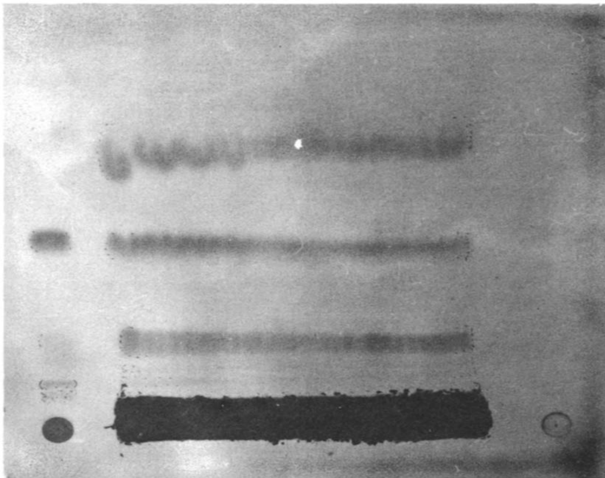
Fig. 1. Chromatographic separation of the lipid constituents of the adrenal extract. Solvent: benzene-ether-acetic acid (70:30:1). Detection with iodine vapour. Plate coated with a 0.5 mm layer of silica gel G. Left: reference lipid mixture. Right: cortisone and deoxycorticosterone used as reference standards. Middle (from the bottom): (1) removed band (phospholipids + corticosteroids); (2) two slight bands of diglycerides; (3) cholesterol; (4) triglycerides; (5) cholesterol esters.
